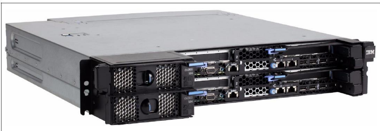
Figure 4-2 Two air-cooled iDataPlex dx360 M4 servers installed in a 2U chassis
