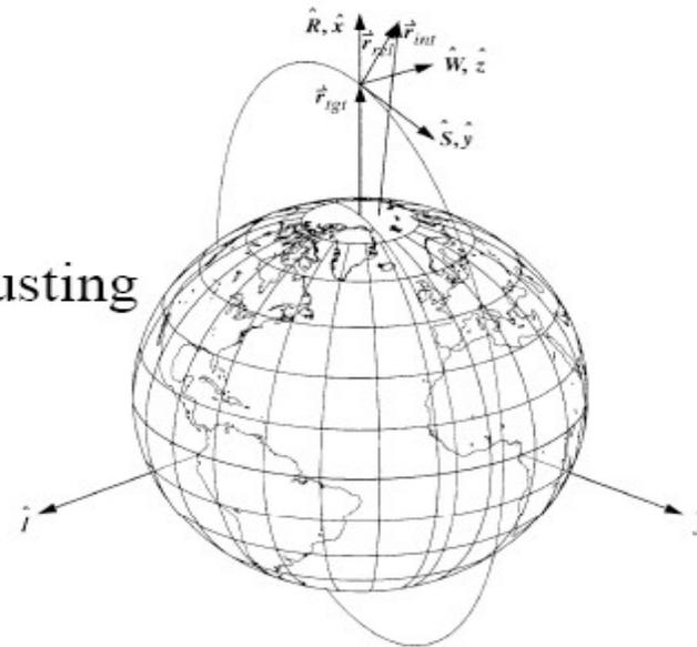
Figure 5-25. Coordinate-System Geometry for Relative Motion. The  $xyz$  notation reminds us the results are approximate. Remember that the  $S$  (and  $y$ ) axes will be aligned with the velocity vector only in circular orbits. A major assumption in relative motion is that the target satellite is in a nearly circular orbit.
