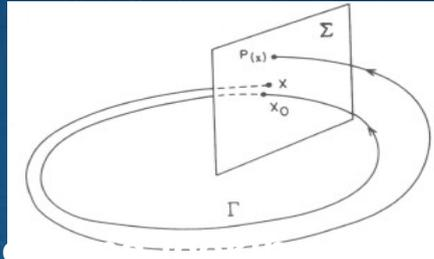
By studying this Poincare section, we can find a stable fixed point, We can find the pseudo-circular orbit (which corresponds to the fixed point in the middle of Figure) whose nearby orbits can be used for formation flight. Clearly, this fixed point corresponds to a periodic orbit in the reduced system.
